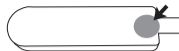
Fig. 3 Apply a small area of thermal compound (not included) to the back of the sensor case where shown
