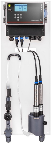
Figure 4. Measurement and control systems are used to determine the residual level of \text{ClO}_2 in the water at a specific sampling point – typically at the end of the loop after the \text{ClO}_2 has reacted throughout the cooling system.
