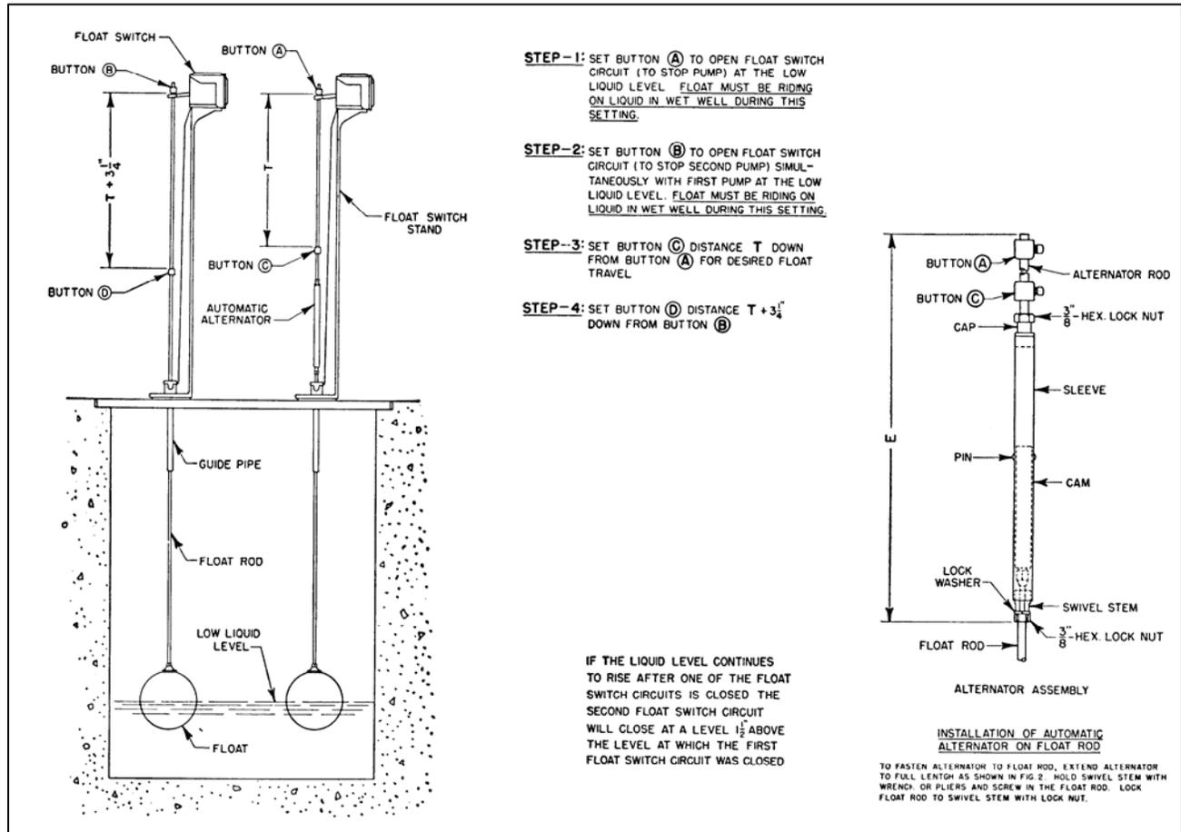
Figure 4 – Installation of Mechanical Alternator
