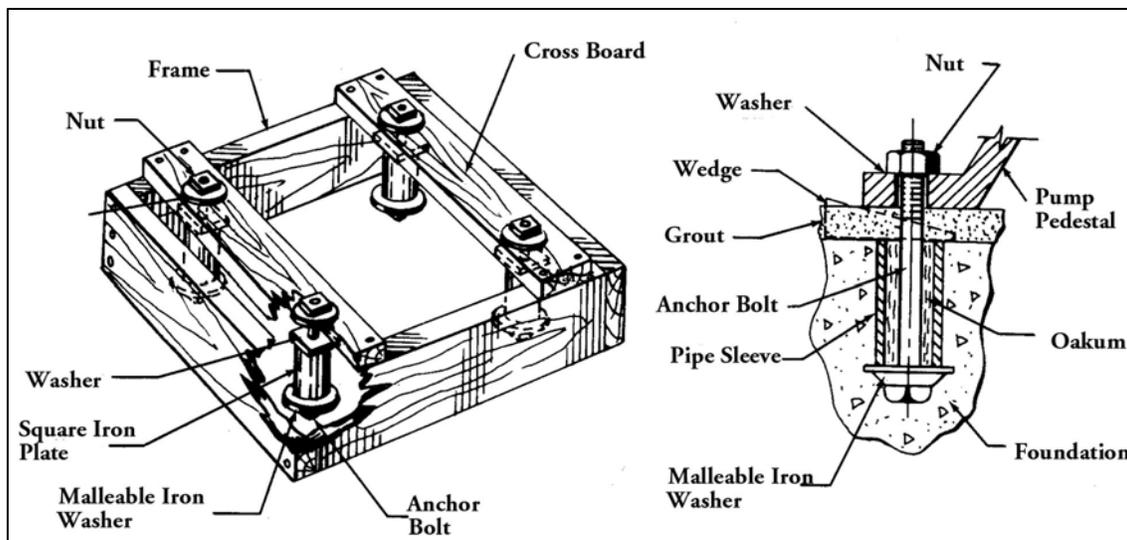
Fig. 2543- A recommended system of foundation Construction
