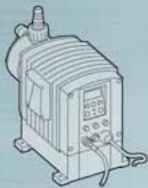
DMS/DME Pump principle: Variable speed diaphragm dosing pump Material: Polypropylene, PVDF and stainless steel Capacity, Q: Min/max. 2.5 ml/h – 940 l/h Pressure, p: Up to 180 bar
