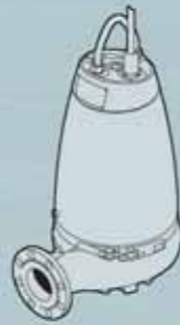
SE1/SEV Pump principle: Submersible, SuperVortex or single channel wastewater pumps Material: Cast iron, stainless steel Flow, Q: Max. 313 m 3 /h Head, H: Max. 45 m
