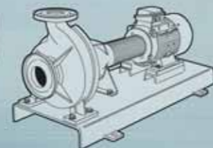
MAXA Pump principle: End-suction process pump, long or close-coupled, electronically controlled as option up to 7.5 kW Material: Stainless steel Flow, Q: Max. 800 m 3 /h Head, H: Max. 97 m
