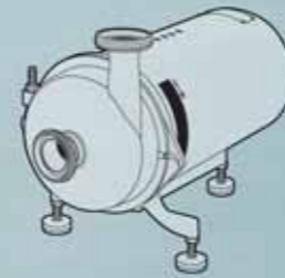
Euro-HYGIA® Pump principle: Single-stage sanitary pump, electronically controlled as option up to 7.5 kW Material: Stainless steel Flow, Q: Max. 130 m 3 /h (250 m 3 /h on request) Head, H: Max. 75 m
