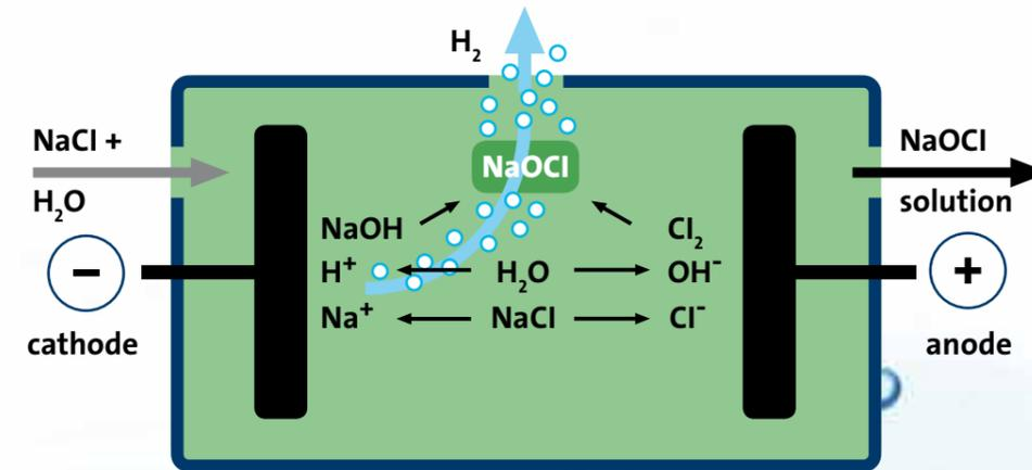
Generation of hypochlorite solution in an electrolytic cell
