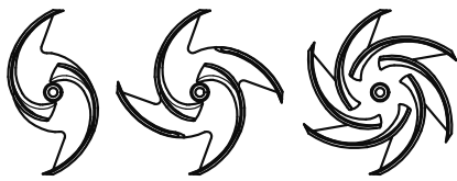
Multiple Vane Impellers Available for different pulp applications.
