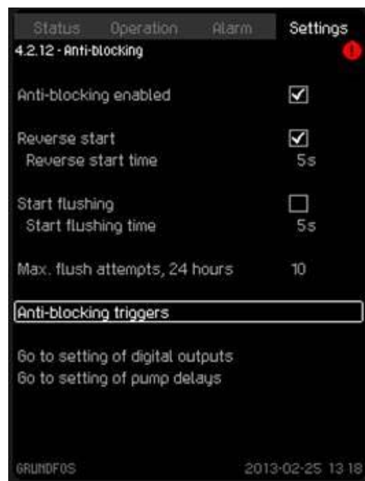
Figure 1) The Grundfos wastewater controller, DC, incorporates anti-blocking protection to optimize
